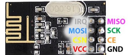
The IRQ pin is only required to be connected if the MY\_RX\_MESSAGE\_BUFFER\_FEATURE is defined in the sketch. Using this feature is recommended for high traffic nodes or gateways.
