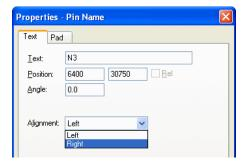
You can change the text alignment that will be used once the symbol is placed in the design and if a pin name has been used, you can opt to align it Left or Right, that is the direction it will read from.
