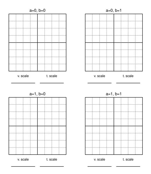
4. For the case in which a=0 and b=1, measure the delay from a transition in c to a transition in f for both fall (tp<sub>HL</sub>) and rising (tp<sub>LH</sub>) edges.
