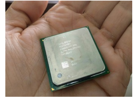
Integrated Circuit Intel Pentium IV (~50Mtt)
