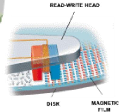
**READ-WRITE HEADS**, attached to the ends of moving arms, slide across both the top and bottom surfaces of the spinning platters. The heads write the data to the platters by aligning the magnetic fields of particles on the platters' surfaces; they read data by detecting the polarities of particles that have already been aligned.
