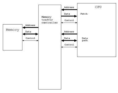
Complete the VHDL description of the Micro6 system architecture provided in the template file system. vhd. The IO unit will not yet be connected in this system. This means that the inputs of the Memory traffic controller that are connected to the IOUnit have to be fixed to zero. Also the direct IO connections from CPU to IOUnit (not shown in above figure) have to be set to zero while the direct connections from IOUnit to CPU have to be left unconnected (also not shown in above figure).
